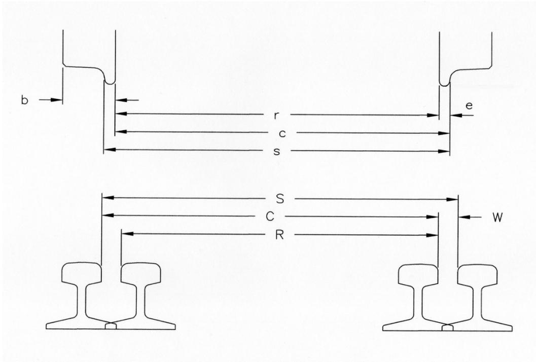
Figure 4 - Critical dimensions for track and wheelsets
