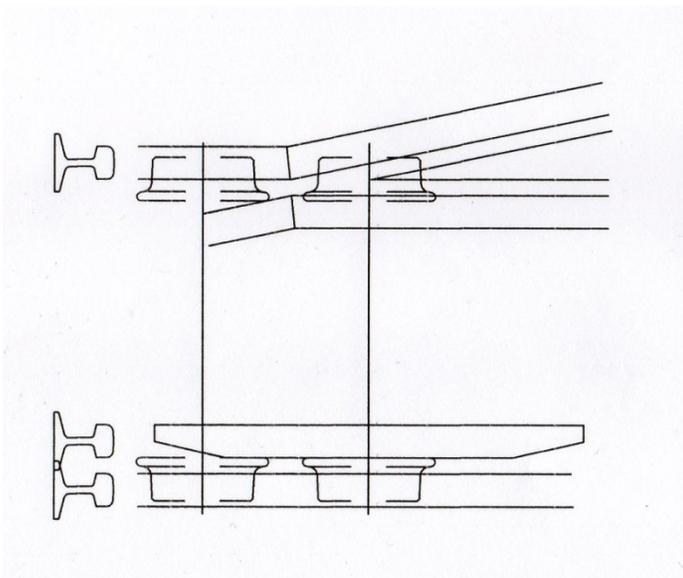
**Figure 3 - The effect of the wheelset being excessively under-gauge (or the check rail being excessively over-gauge). Instead of passing through the crossing flangeway, the flange rides up the wing rail.**
