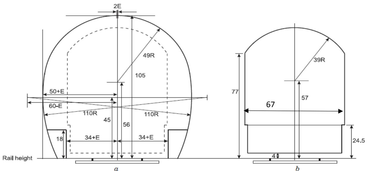
Figure 6 **Limiting Dimensions of Structures and Rolling Stock**
