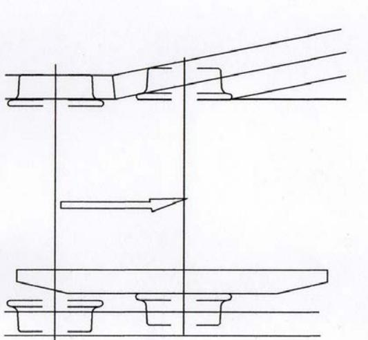
**Figure 2 - The effect of the check rail being under-gauge (or the wheelset being over-gauge). The check rail can no longer hold the opposite wheel flange clear of the crossing gap, resulting in the crossing nose being struck and the wheel derailed.**
