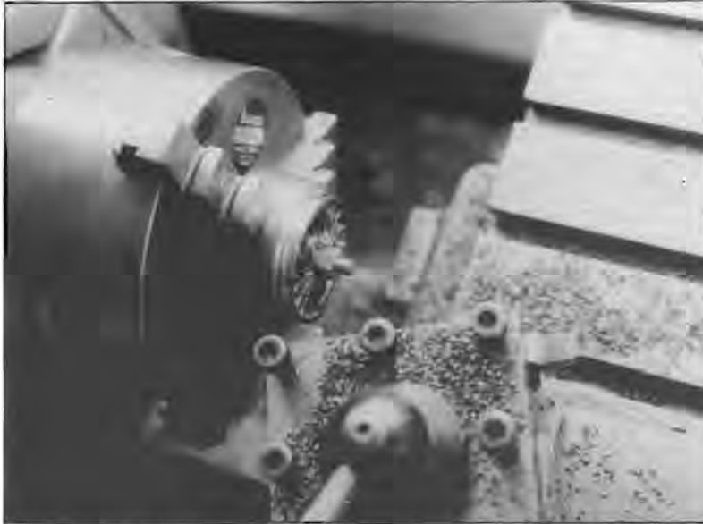
Photo 4.6 The wheel mounted on the special mounting backplate for tread turning. (Photo T. Hughes).
