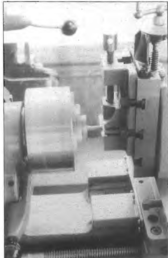
Photo 4.2 Milling the back of the angle after sawing it off the main workpiece. (Photo T. Hughes).
