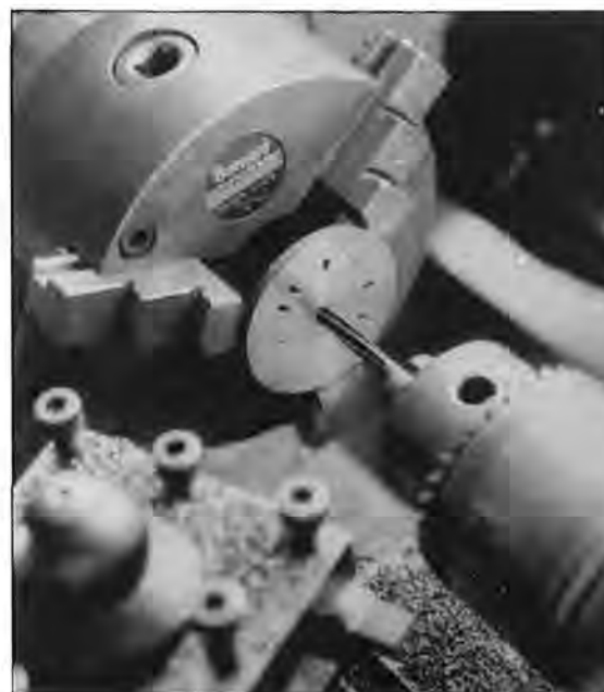
Photo 4.5 Reaming the axle hole in the backed off wheel. Note the spoke holes just showing. (Photo T. Hughes).
