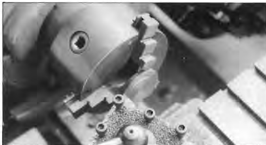
Photo 4.4 A driving wheel casting held in the three jaw chuck while the back is faced off to expose the spokes. (Photo T. Hughes).
