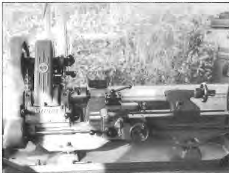
Photo 3.5 A Myford ML7 lathe - no longer produced but occasionally available second-hand. Now superseded by the ML10 and the Super 7. Lathes about this size are ideal for live steam work. (Photo T. Hughes).
