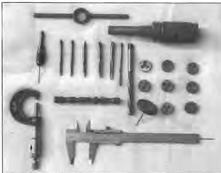
Photo 3.3 Taps and Dies. A die stock, pin vice with 10BA tap, a range of taps and reamers, tailstock die holder, range of dies, Meccano wheel tap holder with 12BA tap, tap wrench, 0-1in micrometer, 0-6in combination vernier. (Photo T. Hughes).
