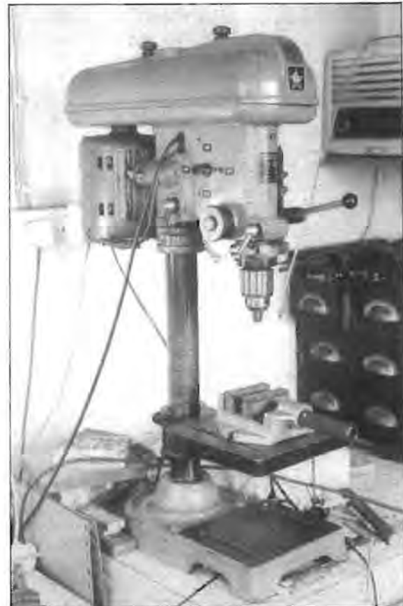
Photo 3.7 A Fobco Star bench drill with 0-1/2in chuck and speed range from 425 rpm. Drills of this type are a useful addition to the workshop. (Photo T. Hughes).
