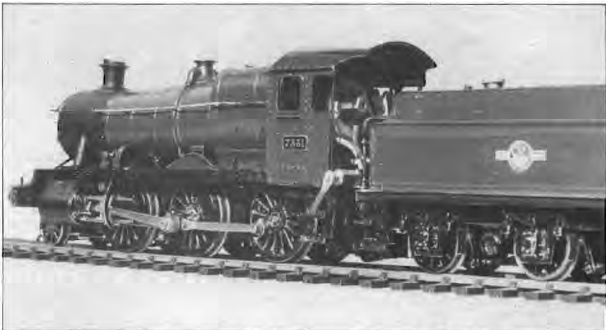
Photo 3.4 A live steam Mogul by the late Fred Eggleton. Except for finished wheels all Fred's locomotives were built entirely by hand using the minimum of equipment. His only 'machine tool' was a hand drill. Nevertheless they turned in some excellent performances. (Photo C. Edwards collection).
