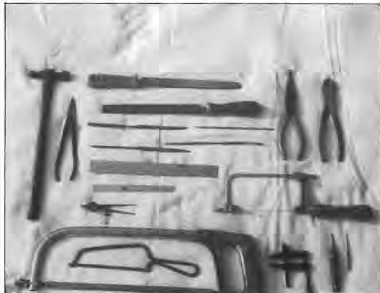
Photo 3.1 A selection of hand tools including a 4oz hammer, tinsnips, coarse flat and fine half-round files, a selection of needle files, long nose pliers, side cutters, combination rule, 6in rule, piercing saw, spring bow dividers, 12in hacksaw, junior hacksaw, toolmaker's clamps, spring loaded centre punch and scriber. (Photo T. Hughes).
