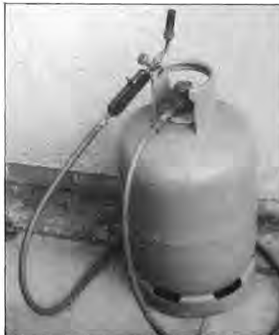
Photo 3.8 A Sievert propane self-blowing gas blowtorch. Various burner nozzles are available to suit a wide range of work. (Photo T. Hughes)
