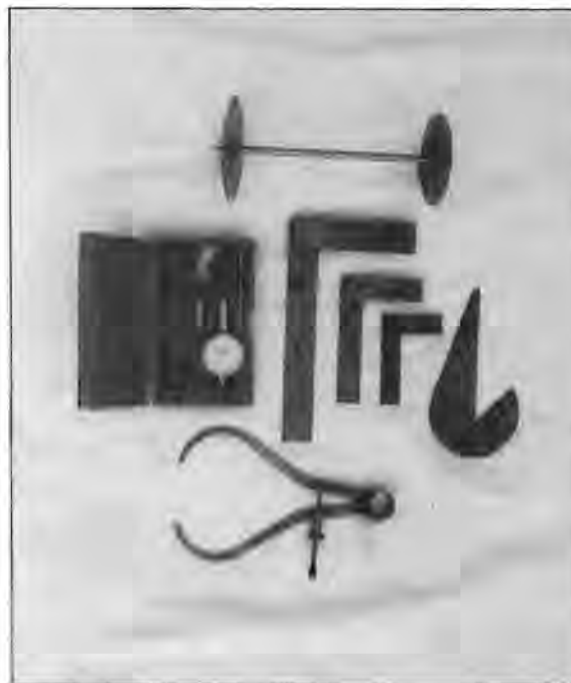
Photo 3.2 Marking out tools. A centre square, 2in, 4in, and 6in try squares, callipers, clock gauge and a 'mystery object': an ingenious home-made device for setting out the shape of a tapered boiler on a flat sheet. The two discs are turned to the boiler diameters at each end of the taper and the distance piece is the length between them. By covering the edge of the discs with marking fluid and rolling them over the sheet the curved outline produced will give the correct taper when cut out and rolled up. (Photo T. Hughes).
