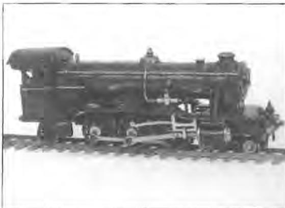
*Photo 1.3 Maerklin 4-6-2 express locomotive for O Gauge but hopelessly out of scale; nearer Gauge 1. Piston valves driven by eccentrics located on the centre drivers. Purchased in Gamages (London) in 1930. Spirit fired. (Photo M. Goodwin).*
