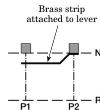
Construction of a single slip is similar to a double slip but, unlike the double slip, the points must be operated in a set sequence to avoid cross feeds. As shown, the route set is from A to D with crossing X1 supplied from the feed side via point P1 switch and crossing X2 supplied from the return side via point P2 switch. This would be considered the normal setting. Reversing P2 sets the route from C to D and connects crossing X2 to the feed side via P2 switch.
