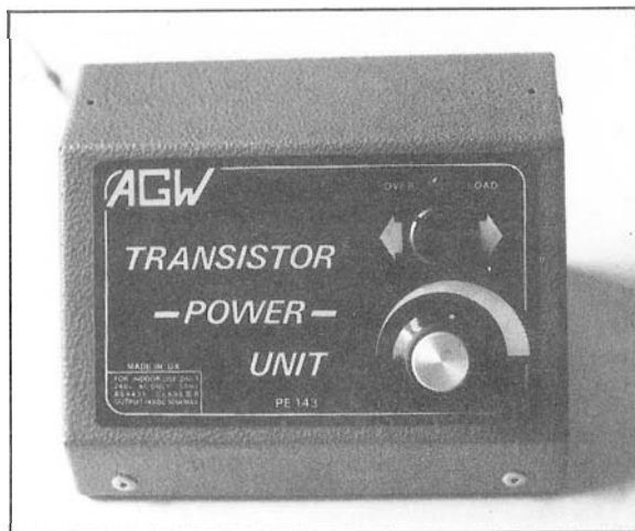
Photo 2.2 A mains fed controller. This one by AGW is rated at 14V 10VA and while satisfactory for 00 scale motors is only suitable for light current motors in O gauge
