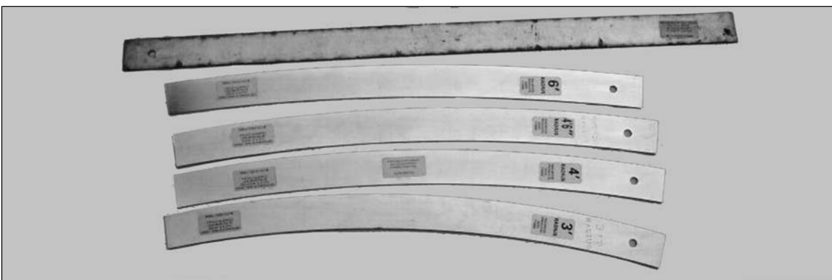
Photo 2.40 The templates illustrated are of laser cut steel and are 32mm wide. They come in a range of radii and are useful both to draw the curves and to aid assembly of track and pointwork
