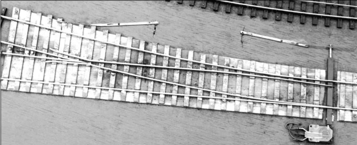
Photo 2.38 Close up of the two rail version. The micro-switch controls the crossing polarity.
