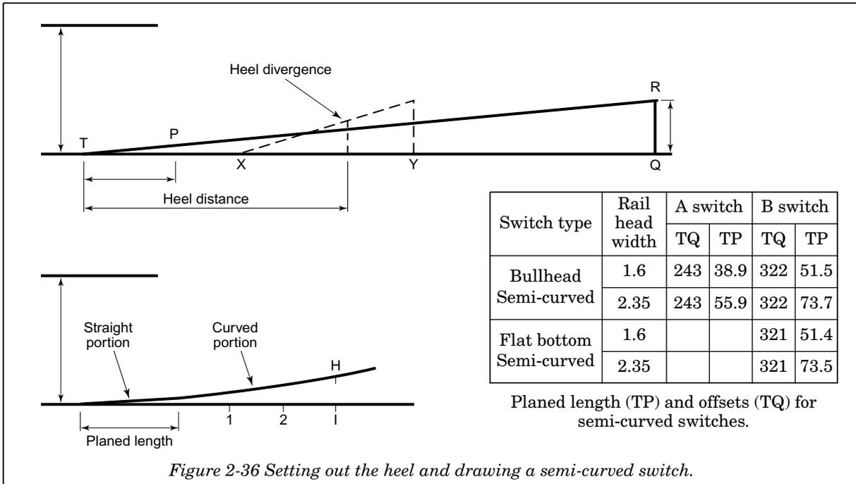
Figure 2-36 Setting out the heel and drawing a semi-curved switch.
