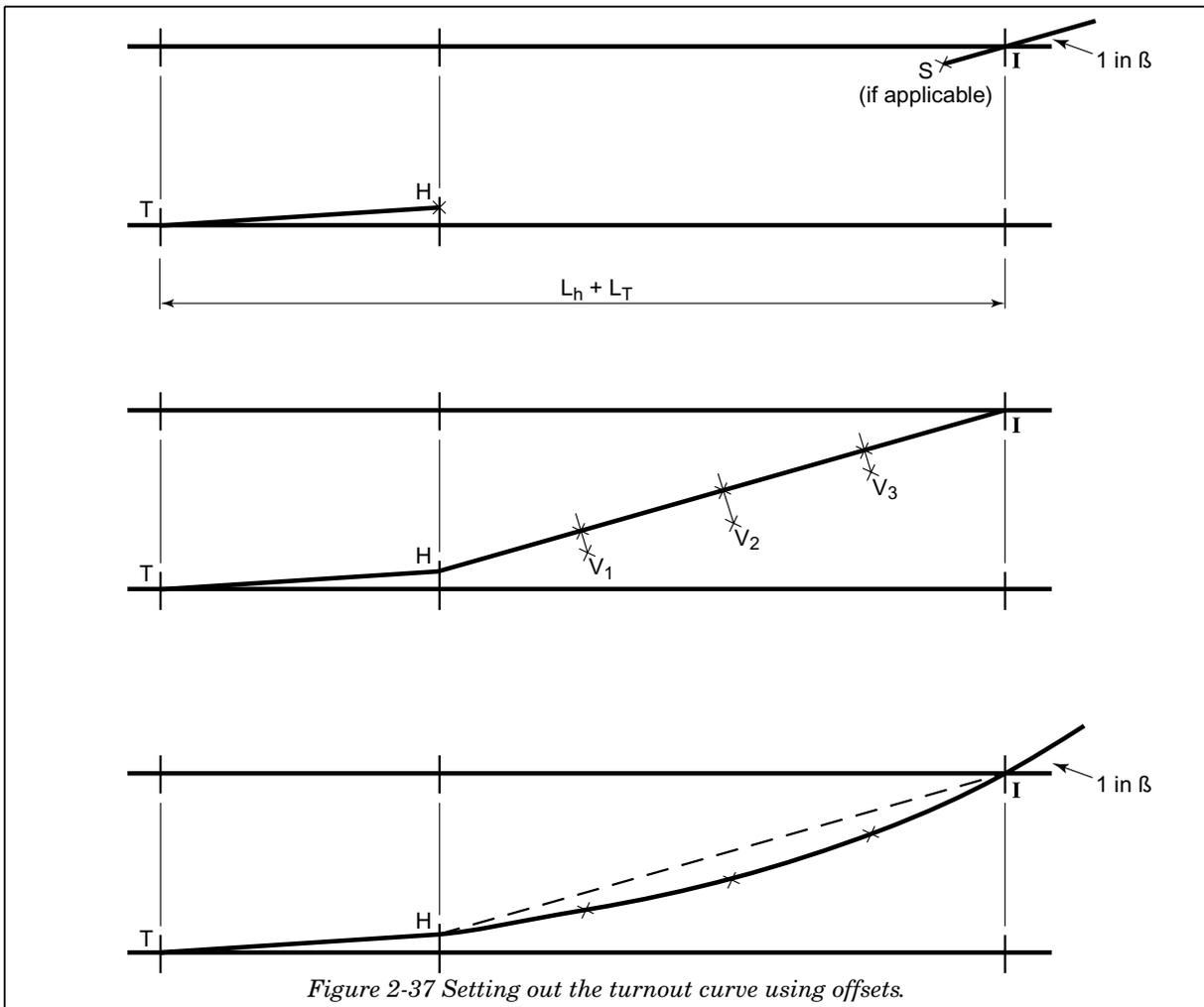
Figure 2-37 Setting out the turnout curve using offsets.
