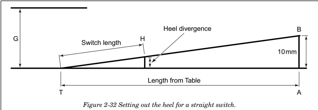
Figure 2-32 Setting out the heel for a straight switch.
