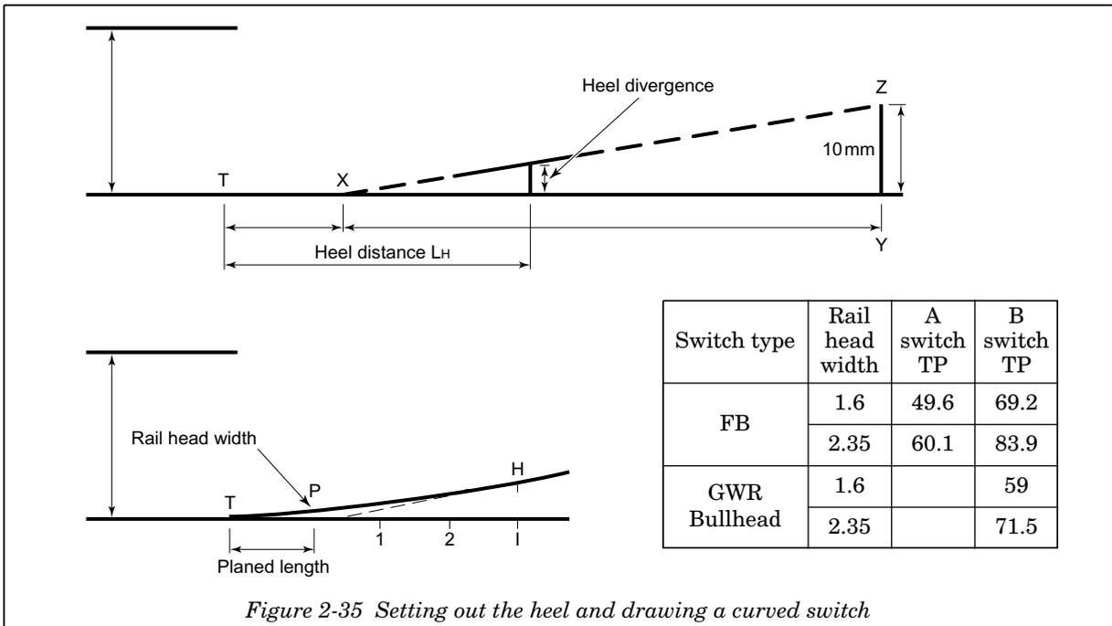
Figure 2-35 Setting out the heel and drawing a curved switch
