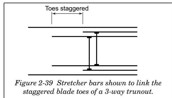
Figure 2-39 Stretcher bars shown to link the staggered blade toes of a 3-way turnout.
