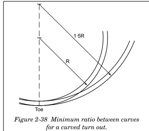
Figure 2-38 Minimum ratio between curves for a curved turnout.
