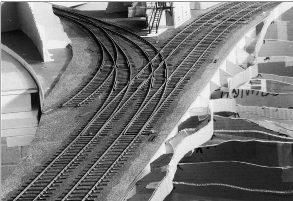
*Photo 2.28 Moorwood Junction – Derby Museum layout. Note the similarity to the Balfour Beatty formation (Photo 2.26) with a continuous curve through the diamond. The treadle for the facing point lock is just visible in the left hand line. The actual lock has not been modelled as its protective cover will hide its location when the scenic work is completed.*
