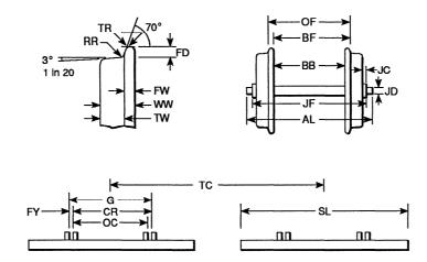
The minimum back to back (BB) dimension must be greater than the maximum dimension over the check rails (OC). The maximum back to flange face dimension (BF) must be equal to or less than the minimum check rail to opposite rail face dimension (CR). The minimum wheel width (WW) must be equal to or greater than twice the minimum flangeway (2FY).
